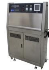
UV lamp aging test chamber
